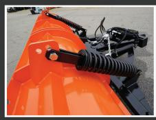
3 way adjustable trip springs for desired angle of attack
